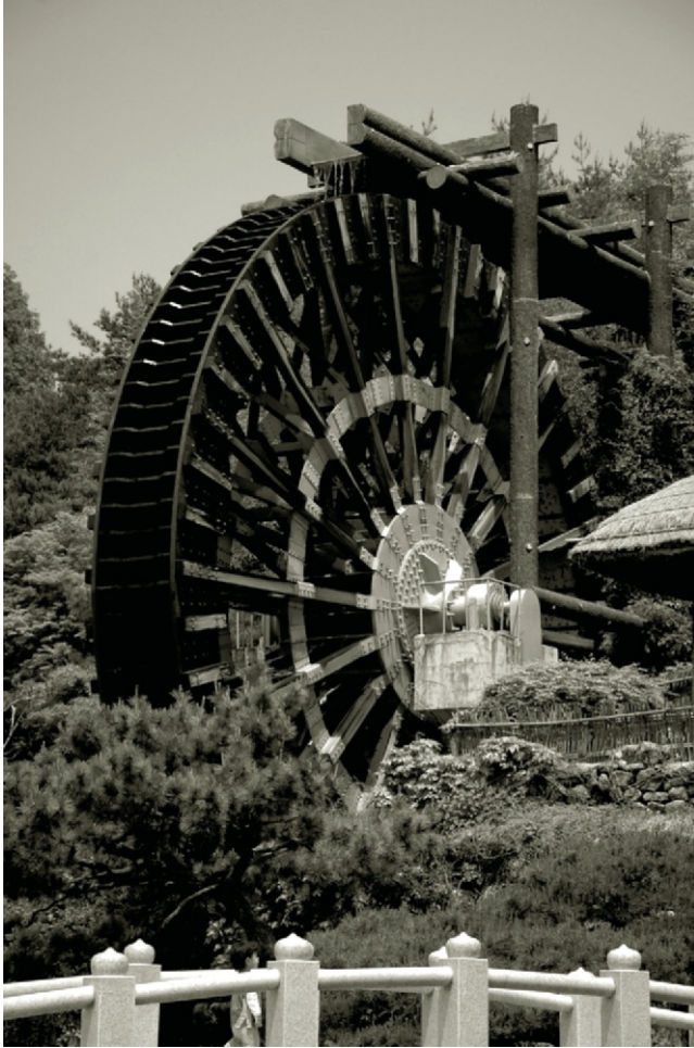
Figure 2.18i An overshot waterwheel is best used where river water can be diverted high enough to be dropped onto the waterwheel. The waterwheel shown is in Korea.
