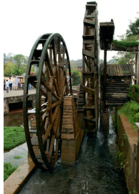
Figure 2.18j Undershot waterwheels use the flow of the river for power. These Chinese waterwheels were used to lift river water for irrigation.
