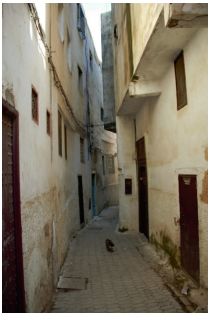
Figure 17.2a This narrow alley in the old section of Fez, Morocco, provides much shade for the windows, walls, and the alley itself. The white walls further reduce solar heat gain.
